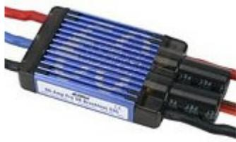
While using more than 3 Lithium cells may require the use of a separate receiver battery on some ESCs, the new 60-Amp [Pro SB Brushless ESC](#) with Switch-Mode BEC allows you to operate up to 7 analog or 6 digital standard-sized servos with the BEC on any recommended input voltage from 3s to 6s LiPo.
