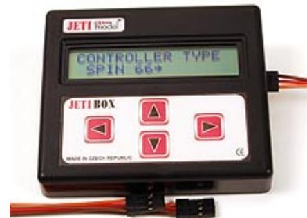
The key things to know are that the longer cable with the (+ - and signal label) symbols on it connects to the ESC and if you are using an OPTO controller, a separate
