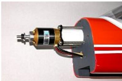
The AXI line of outrunner motors has several selections in this 400 watt class, the heavier 4120 motor for 4-5 LiPo cells, and, the lighter 2826 for 3-5 LiPo cells. The AXI motors are direct drive brushless designs that are virtually maintenance-free. Since there are no brushes to wear out and no gears to lubricate or strip, the motors need no maintenance other than perhaps a yearly lubrication of the ball bearings supporting the drive shaft.
