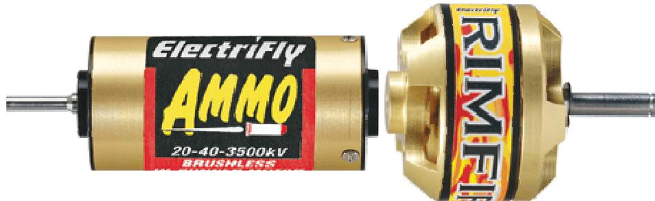
The ElectriFly AMMO motor on the left is an inrunner. The outside can is stationary and it only spins the shaft on the outside of the motor. Typically, but not always, this type of motor requires a gearbox which allows them to swing larger props efficiently. Some inrunners, especially the brushless kind, can spin a larger prop directly without the need for a gearbox. On many inrunners, when a gearbox is not used, only a small prop can be used that spins very fast.
