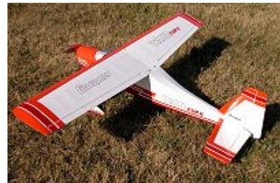
Using the middle of our rule of thumb power level for trainer-type planes, we multiply 65watts times 6lbs to get 390 watts which is about 1/2 h.p. The result of about 400 watts is the motor class that we need to select from for our conversion project.
