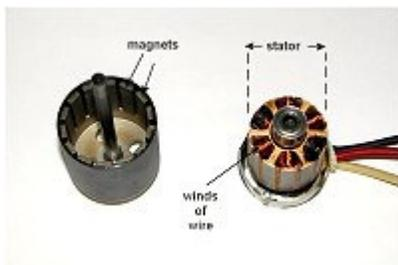
Most outrunners use a 6-digit numbering system like the AXI 5330/18. The first two numbers (53) represent the diameter of the stator in millimeters. The stator is the fixed part in the middle of the motor. The second two numbers (30) represent the length of magnets in millimeters. These long rectangular magnets are attached to the inside of the rotating case. The third set of two numbers (18) represents the number of wire winds, also called turns.
