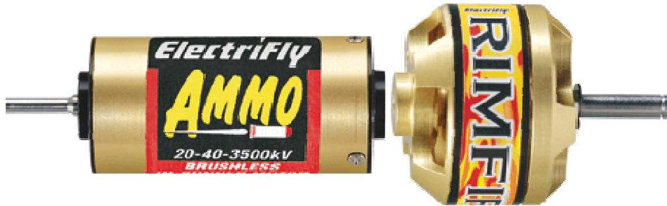
The ElectriFly AMMO motor on the left is an inrunner. The outside can is stationary and it only spins the shaft on the outside of the motor. Typically, but not always, this type of motor requires a gearbox which allows them to swing larger props efficiently. Some inrunners, especially the brushless kind, can spin a larger prop directly without the need for a gearbox. On many inrunners, when a gearbox is not used, only a small prop can be used that spins very fast.
